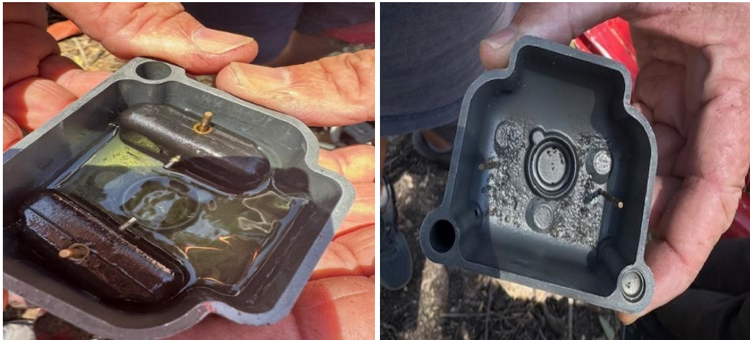
Figures 15 and 16: The left side carburettor showing water contaminated in the float bowl (left picture). Corrosion at the bottom of the right carburettor float bowl (right picture).
