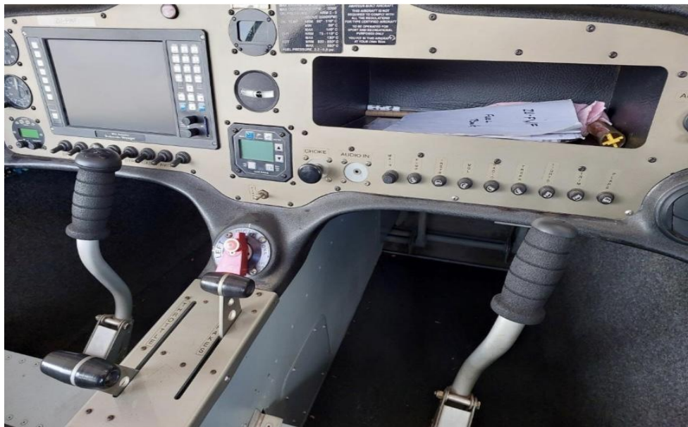
Figure 4: The ZU-FWF cockpit showing the Stratomaster Voyager MGL Avionics EFIS.
