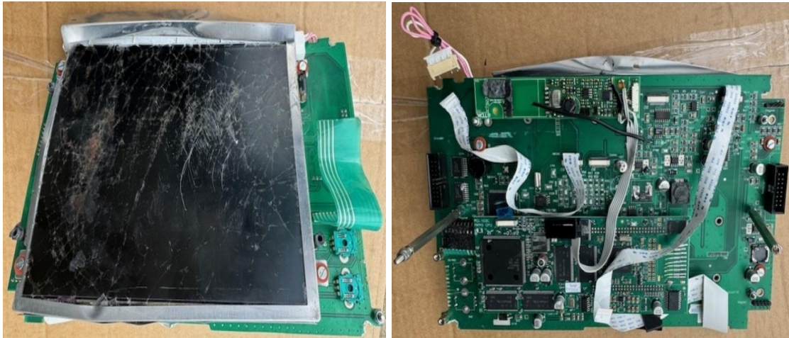
Figures 5 and 6: The EFIS unit (back and front) after it was removed from the cockpit.
