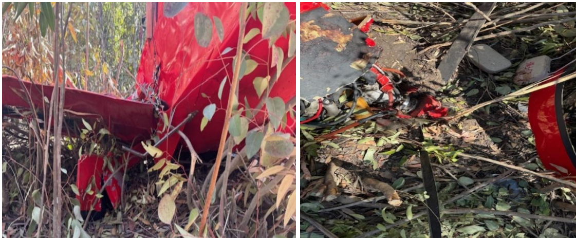
Figures 12 and 13: The left wing with the flaps retracted (UP position) and the left main gear strut that has stretched backward. The engine nose section is buried under the soft ground, and the remaining two blades are still intact.
