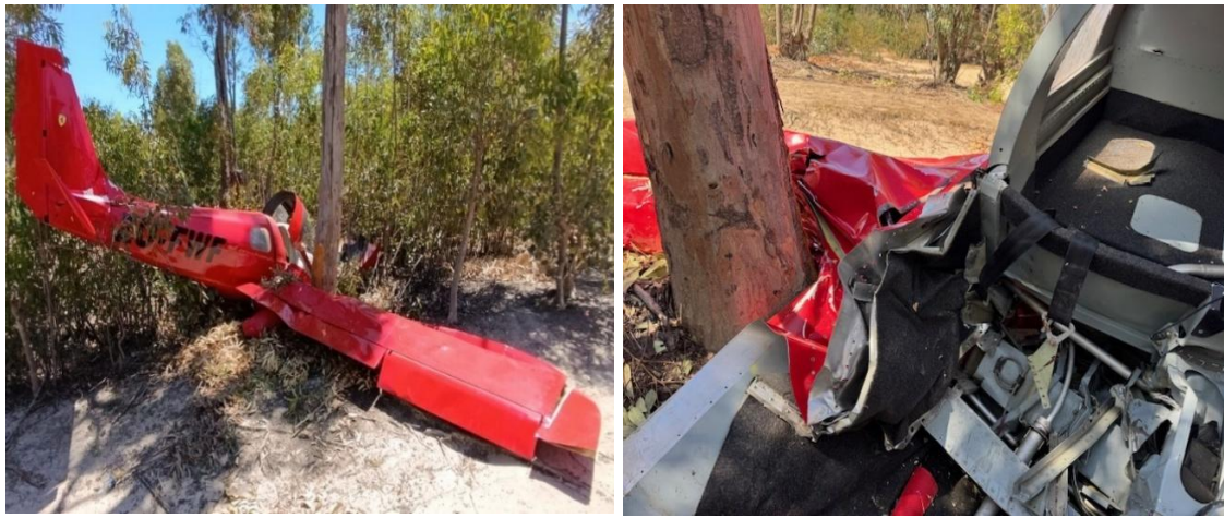
Figures 10 and 11: The aircraft's right-wing root against the tree stem.
