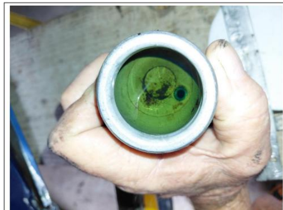
Figure 6: Small fragments of rubber were found in the left-side fuel filter.
