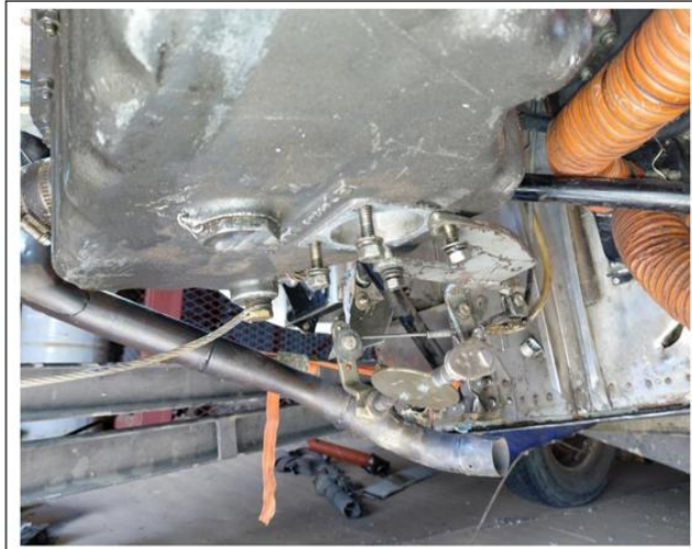
Figures 2 and 3: The bottom part of the engine showing carburettor mounting position (left); and the damaged carburettor after the accident (right).
