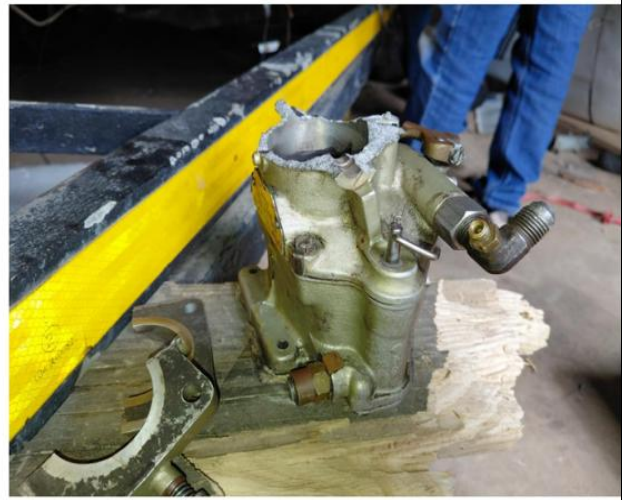
Figures 2 and 3: The bottom part of the engine showing carburettor mounting position (left); and the damaged carburettor after the accident (right).
