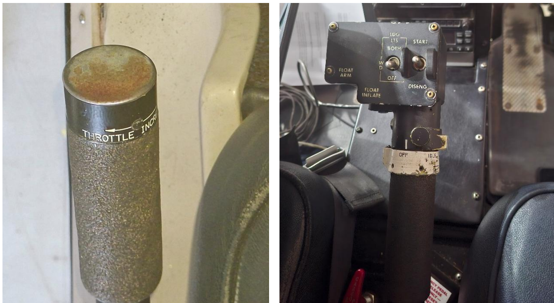
Figures 5 and 6: The auxiliary throttle on the left-side pilot seat (left). The throttle for the pilot seated on the right seat (right).
