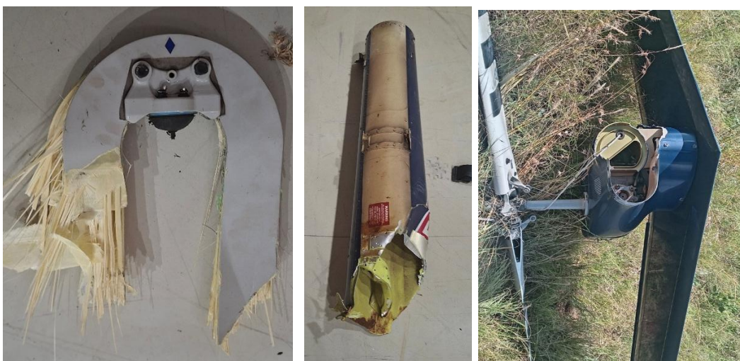
Figures 2, 3 and 4: The rotor blade that broke off (left), and the tail boom and tail rotor that were severed during the accident (centre and right). (Source: Operator)
