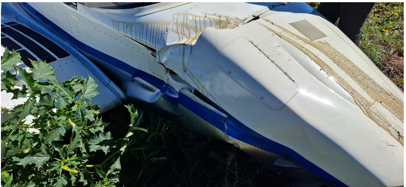
Figure 2: The spilled oil on the aircraft. (Source: Pilot)
