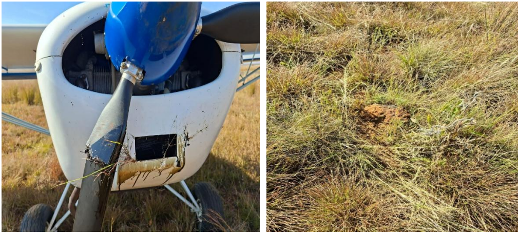
Figures 3 and 4: The damaged propeller blade (left picture), and the impacted anthill (right). (Source: Pilot)
