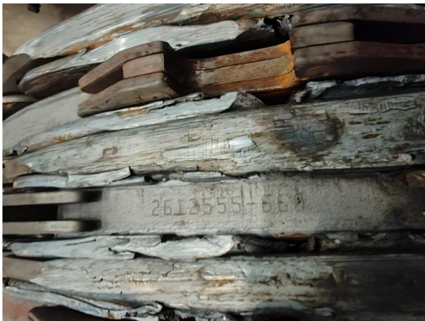
Figure16: The left main landing gear outboard brake unit shows galling damage and material transfer.
