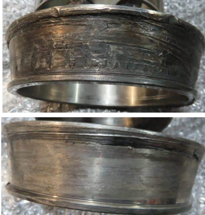
Figures 9 and 10: The bottom half of the outboard bearing cone with high heat indications and roller indentations and scoring; and the top half of the outboard bearing cone with no high heat indications and roller indentations and only showing mechanical damage from roller scoring.
