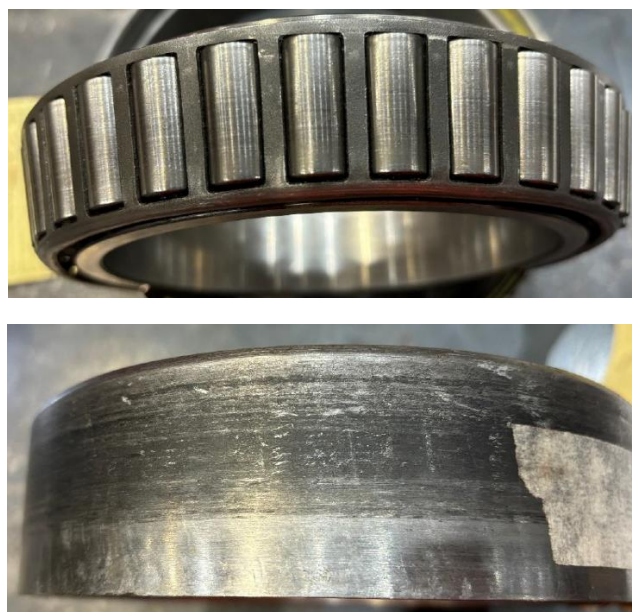
Figures 11 and 12: The inboard with the cone intact (top) and the inboard bearing sleeve with minor rotational scoring (bottom).
