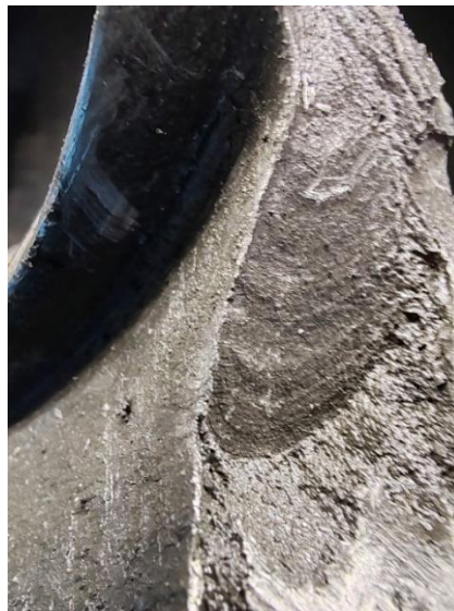
Figure 5: Fatigue crack initiation site at the bearing thrust shoulder.
