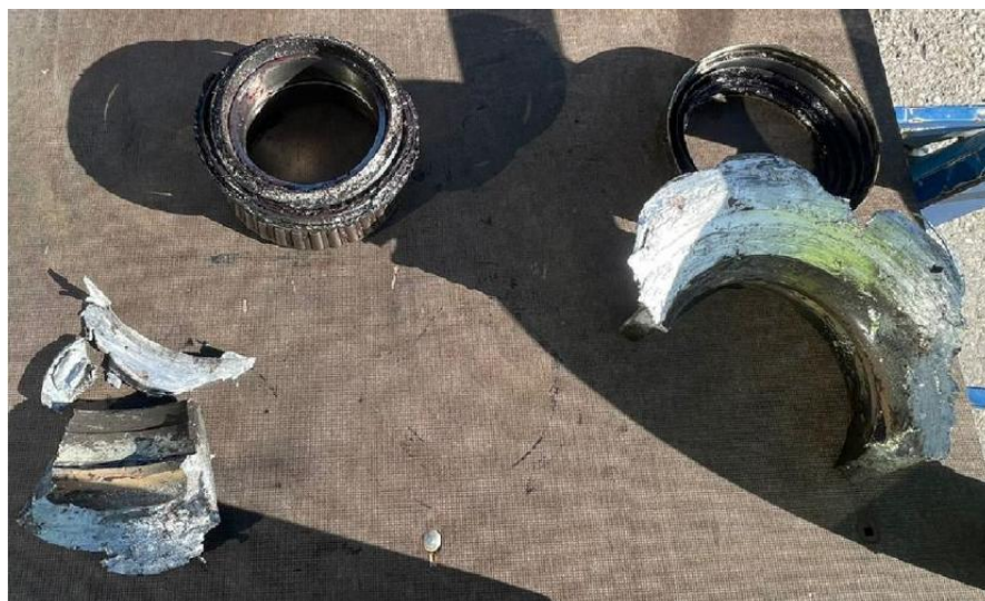
Figure 17: Hub pieces from IN-019/2022 involving RyanAir aircraft.
