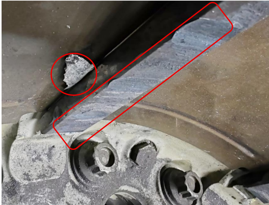
Figure 13: Brake rotor drive key with galling damage and a piece of the failed hub wedged behind it.
