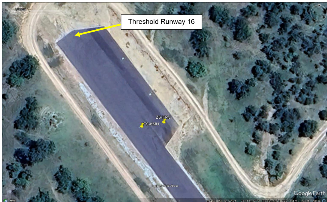
Figure 1: The position of the two aircraft when the wing impact occurred. (Source: Google Earth)
