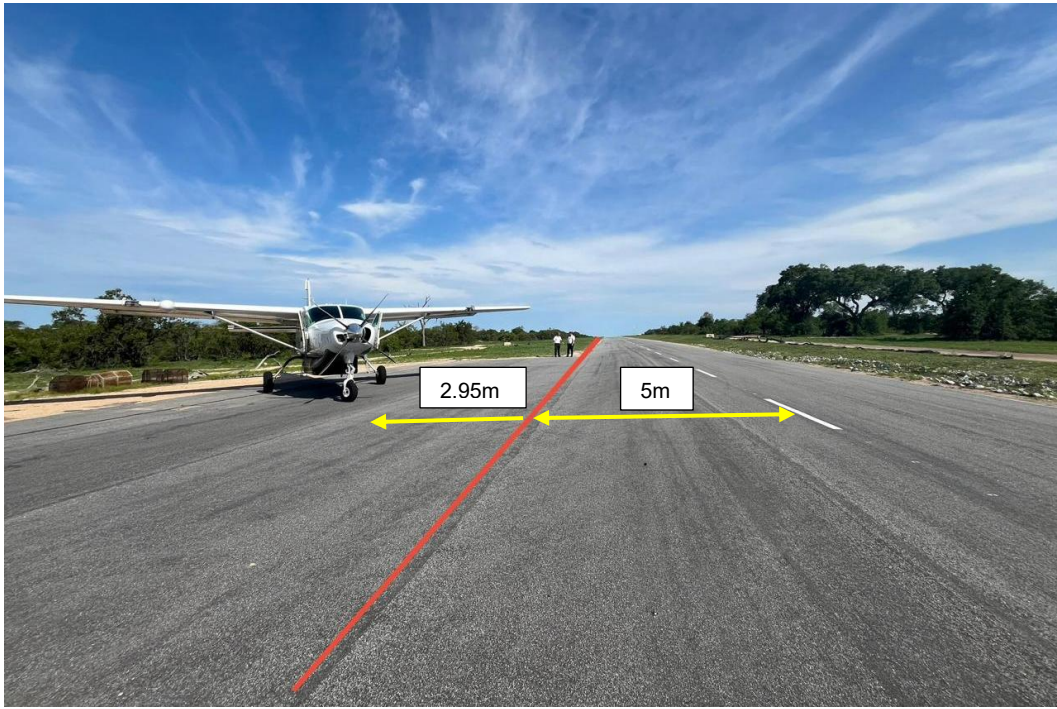
Figure 2: The ZS-KMJ aircraft as it was parked next to Runway 16 at the time. (Source: Operator) The two arrows indicate the distance from the runway centreline to the runway edge which is 5m, and the wing exceeding the runway edge by 2.95m.
