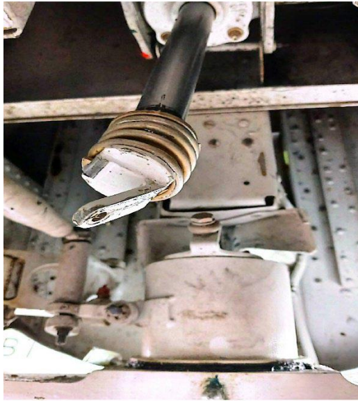
Figures 3 and 4: Damage to the nose gear actuator (left picture) and drag braces (right picture). (Source: Aerotech)
