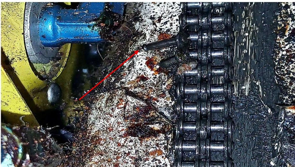
Figure 2: Damage to the duplex chain and the detached link on the floor panel (red arrow). (Source: Aerotech)
