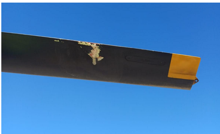
Figure 3: The main rotor blade that struck the top part of the vertical stabiliser. (Source: Operator)
