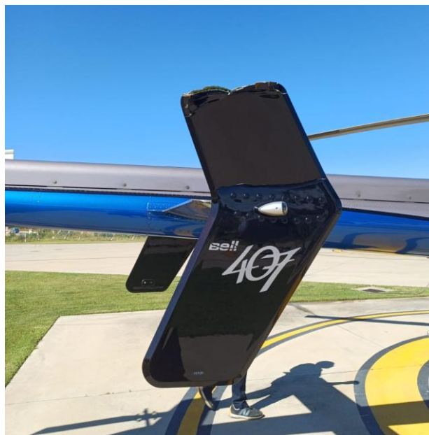
Figures 1 and 2: Damage to the top section of the two vertical stabilisers. (Source: Operator)
