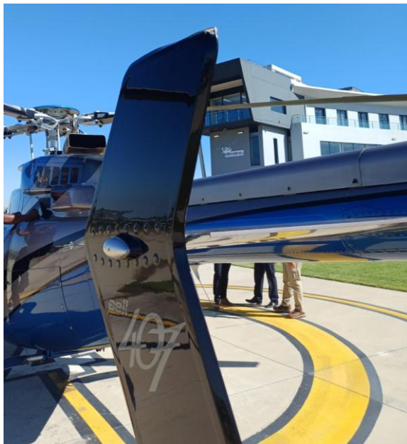
Figures 1 and 2: Damage to the top section of the two vertical stabilisers. (Source: Operator)
