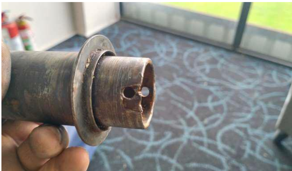
Figure 3: The close-up picture of the failed shear bolt.
