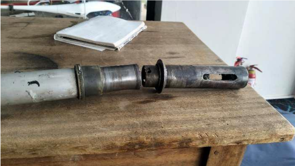
Figure 2: The failed shear bolt.
