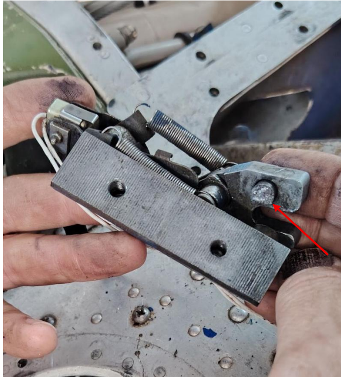
Figure 4: The landing gear down-lock support assembly pin that sheared off.
