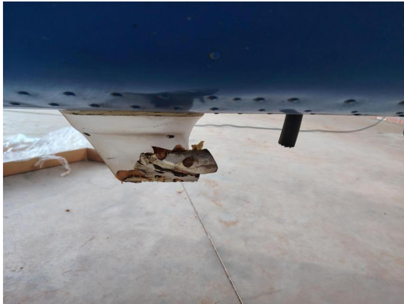
Figure 3: The damaged antenna in the rear fuselage area.
