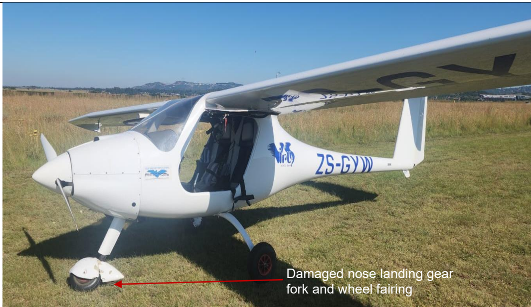
Figure 2: The aircraft with a damaged nose landing gear fork and wheel fairing. (Source: Pilot)
