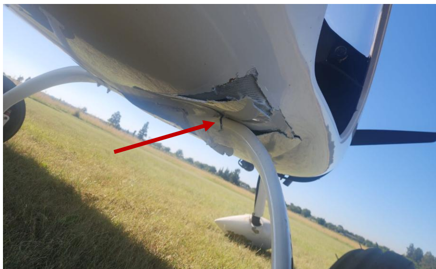
Figure 3: The right main landing gear and the area where the breakage occurred (red arrow). (Source: Pilot)
