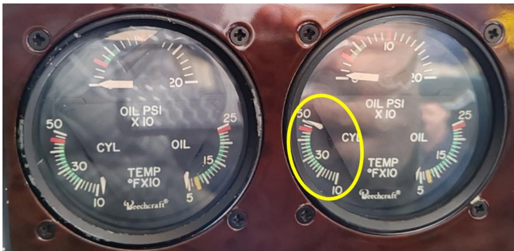
Figure 4: The engine's right-side cylinder head temperature gauge at full deflection with the engine off.
