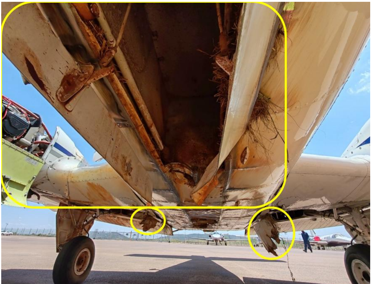
Figure 1: The damaged landing gear doors and belly of the ZS-CHL aircraft.
