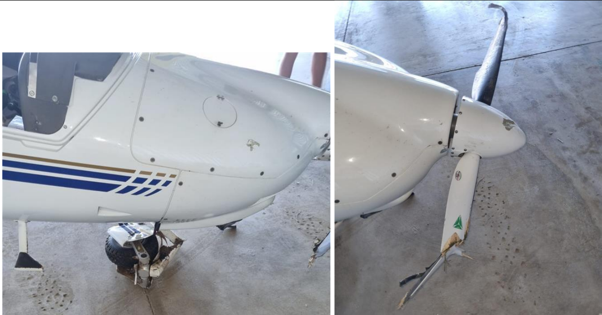
Figures 2 and 3: The damaged nose gear strut (left picture); the damaged propeller blades (right picture). (Source: Pilot)
