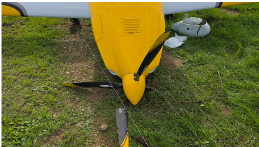
Figure 3: The damaged nose section and the severed propeller blade. (Source: Pilot)
