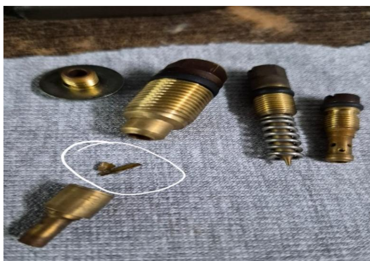
Figure 4: The right carburettor bowl main jet and pieces of what appeared to be PRC sealant. (Source: AMO)
