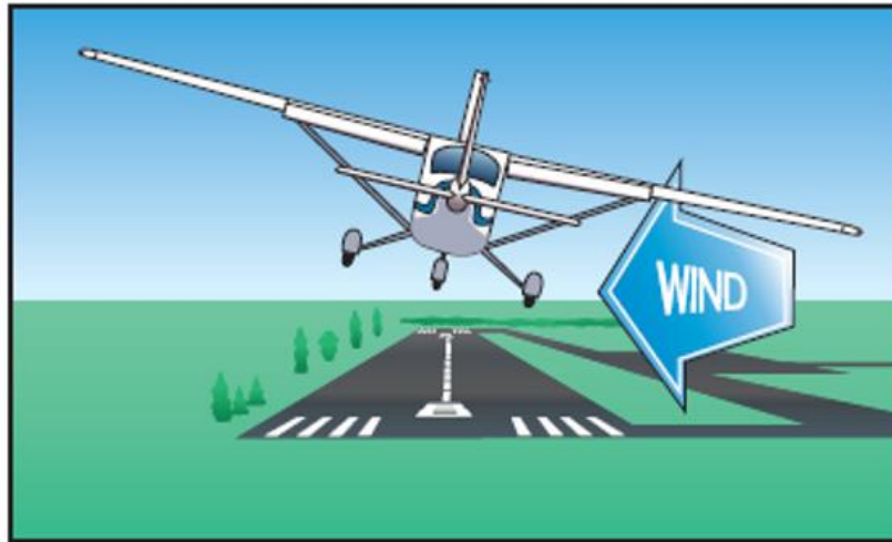
Figure 4: Sideslip technique illustration. (Source: FAA-H-8083-3A)
