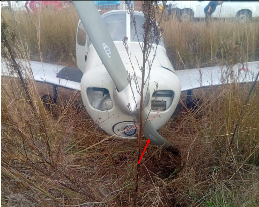
Figure 3: The damaged propeller blade.
