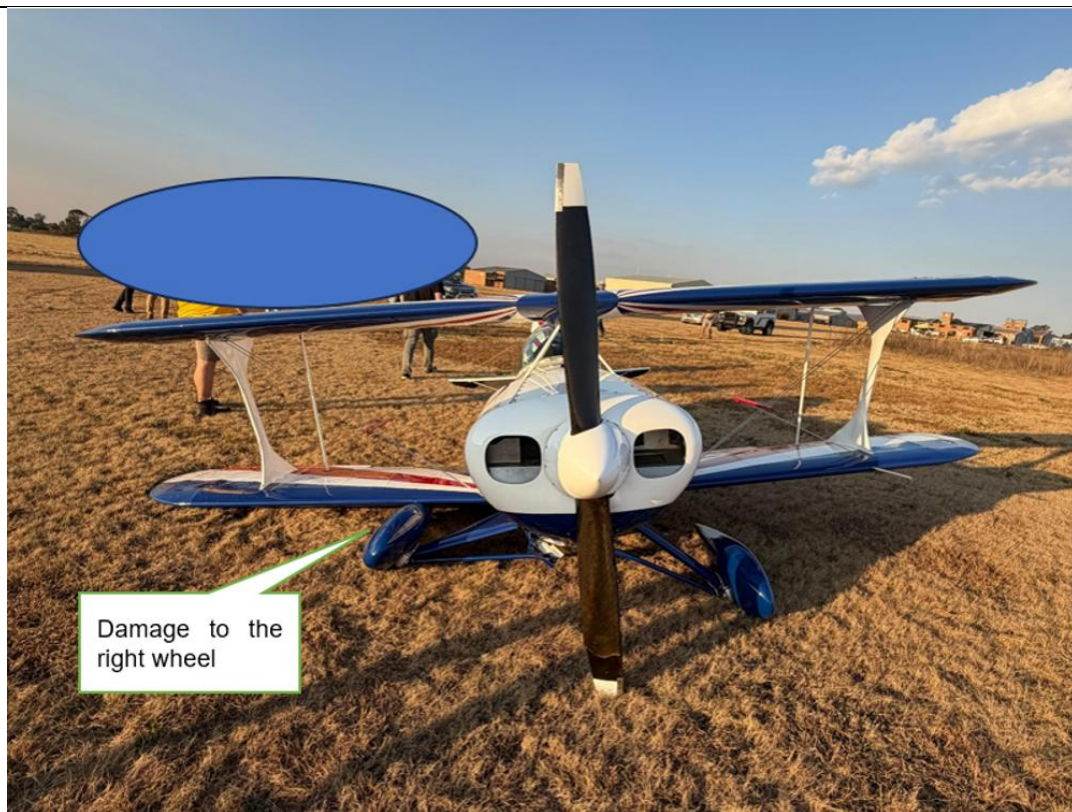
Figure 3: The damaged right wheel. (Source: Pilot)
