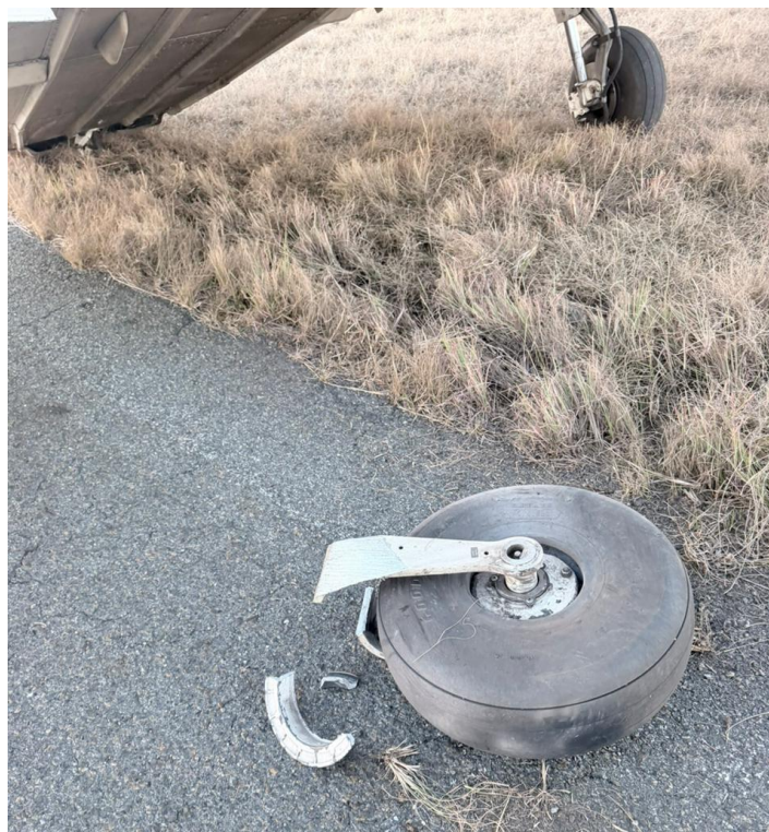
Figure 3: The severed nose gear fork and well assembly. (Source: Operator)
