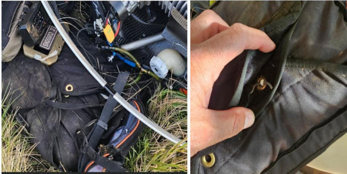
Figure 18: The reserve parachute with one securing pin missing.
