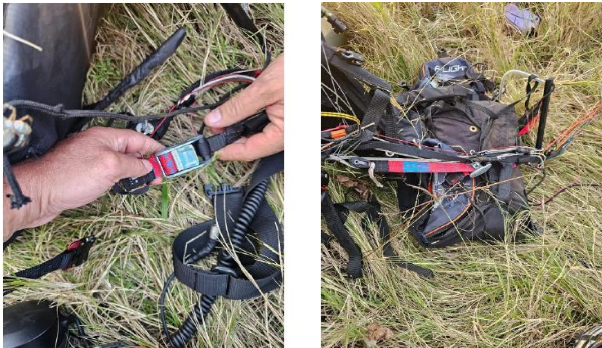
Figure 20: The wing riser trimmers were set to a maximum position No.12 as indicated.
