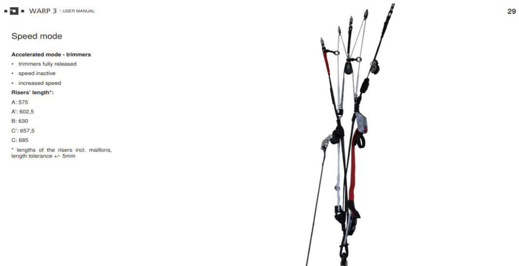
Figure 22: Illustration of the wing speed trim controls.
