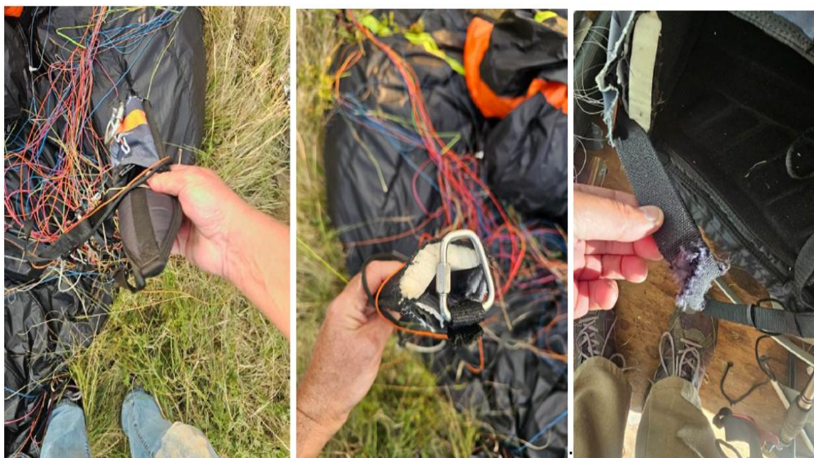
Figure 17: Cut-off harnesses by first responders: shoulder, leg straps and the stomach harnesses.
