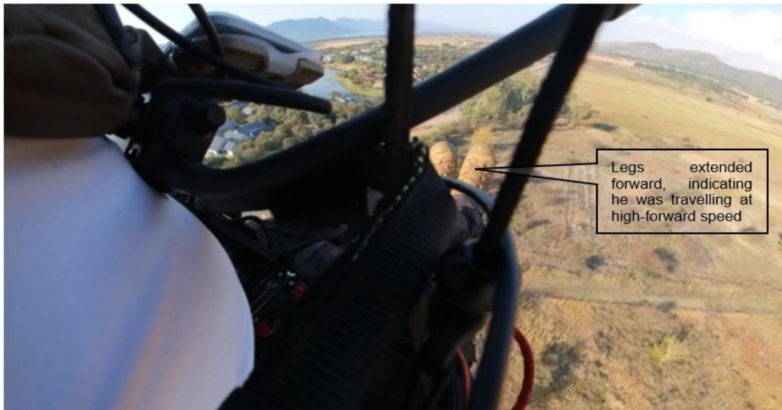
Figure 8: The picture shows the pilot with his legs extended forward, consistent with speed-bar position.
