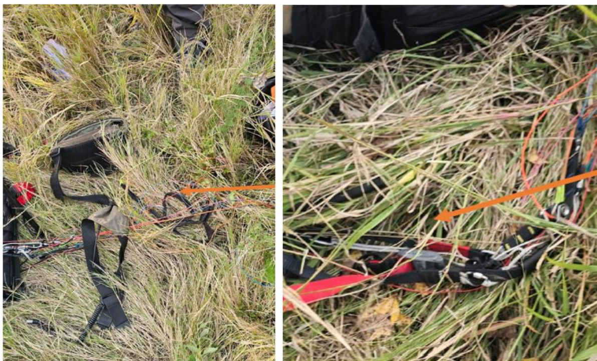
Figure 19: The cut straps, brake handle, wing riser strap and the speed.
