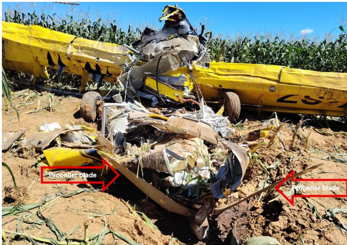
Figure 5: The front portion of the aircraft and the two propeller blades that had remained intact.
