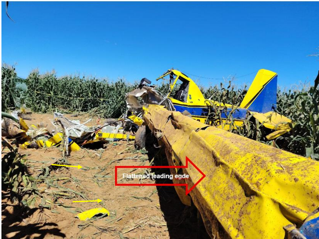
Figure 6: The flattened leading edge of the left wing and the impact mark on the ground (yellow arrows).
