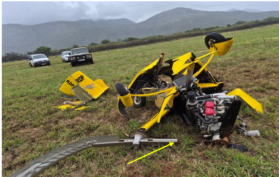
Figure 5: The wreckage at the accident site and the main rotor blade that failed (yellow arrow).
