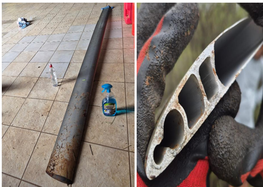
Figures 6 and 7: The portion of the main rotor blade that broke off (left picture). The close-up picture of the blade and the area where it snapped (right picture).
