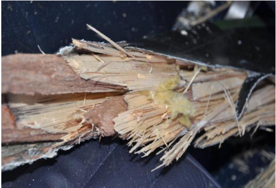
Figure 11: Fragments of the propeller blade.
