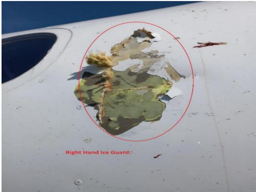
Figure 7: The damaged fuselage.
