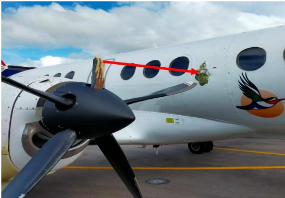
Figure 6: Fragments of the propeller blades penetrated the fuselage.
