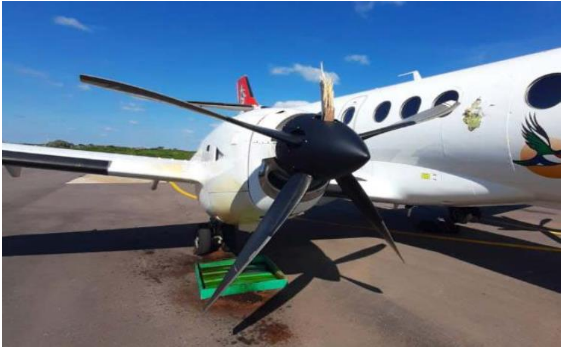
Figure 2: Damage to the propeller.
