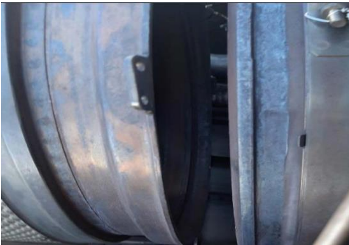
Figure 15: The dislodged combustion casing.
