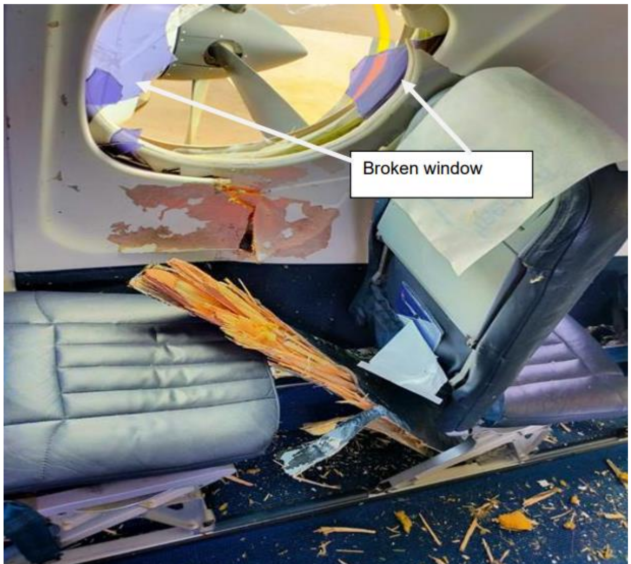
Figure 16: Damage to the third row of seats.
