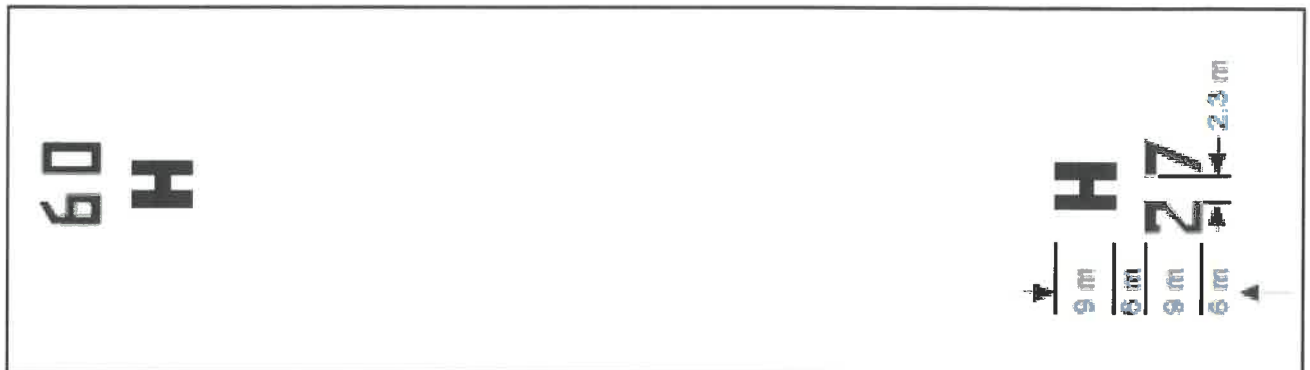
Figure 25. FaTo designation marking and heliport identification marking for a runway-type FaTo
